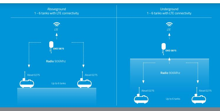
AIUT's Propane Remote Tank Monitoring Solution consists of 2 units: OKO 5875-telemetry unit and ALEVEL 0275-smart tank sensor.
