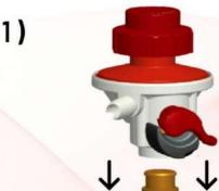
To install, place the regulator over the gas cylinder and press downwards firmly until you hear it clicking into position
