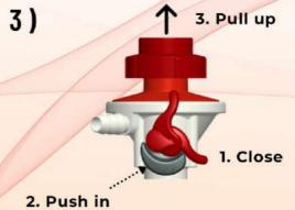
To release, push in the release button and pull up the regulator.
