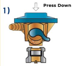
To install, place the regulator over the gas cylinder and press downwards firmly until you hear it clicking into position
