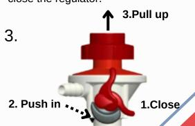
To release, push in the release button and pull up the regulator.
